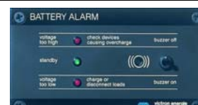
Panel 'Battery Alarm'
